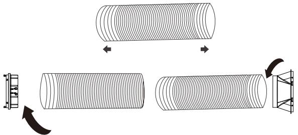
**2. install the exhaust air hose on the unit**
