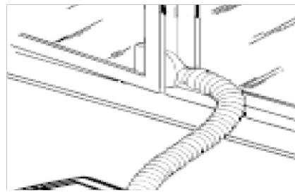
**4. installation on roller shutter and sliding windows using the window bracket**
