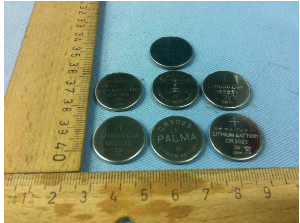
Battery/电池 CR2025 3,0V 150mAh
