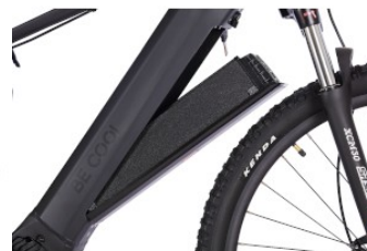
Detailed view of battery
